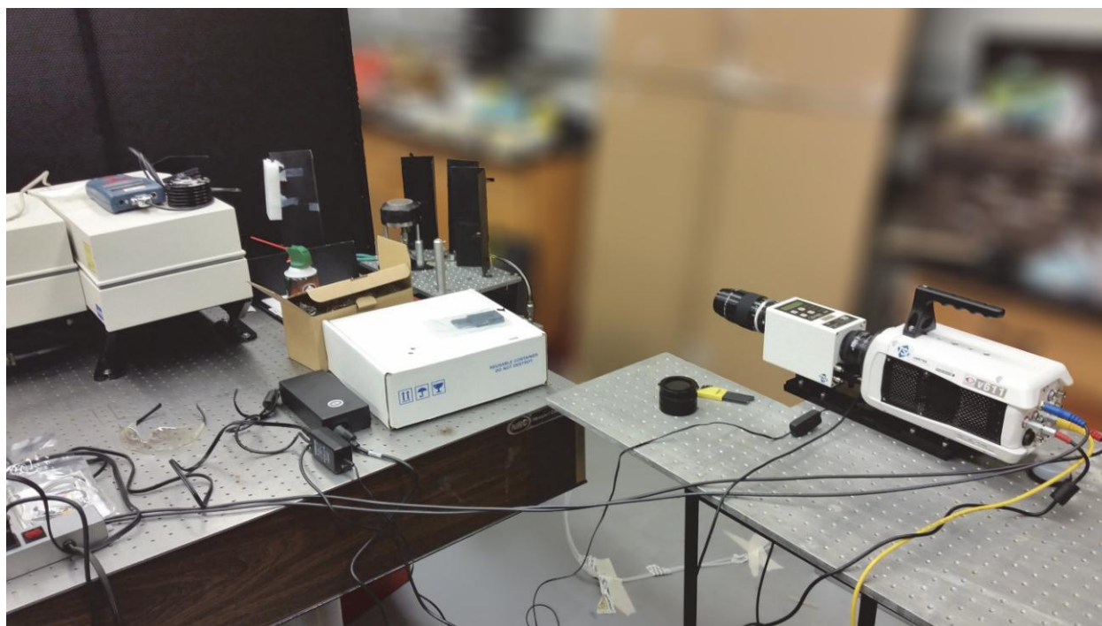
Fig. 1 Experimental setup showing the TSI combustion PLIF system consisting of a dye laser (left), flat flame burner (center left), and camera and intensifier (right).
